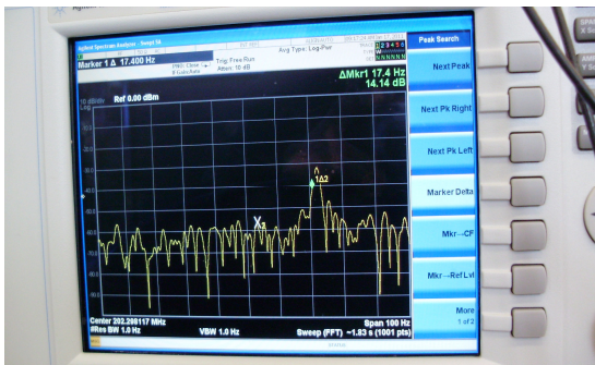
Fig. 9b PLL fractional frequency operation f_c = 200 MHz+ \Delta f , SPAN=100Hz, RES=1Hz
